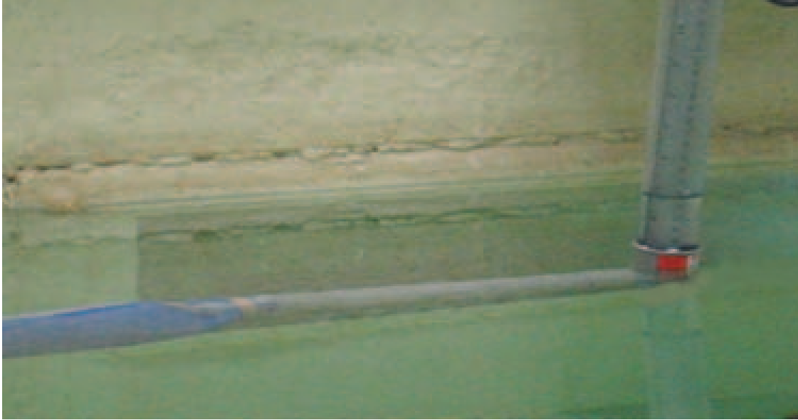
Figure 3. Bulge tube in wave tank with manometer. The waves are coming from the left. Oscillations in the manometer were about 5 times the wave height.
