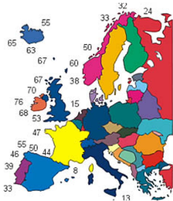
Figure 5. European Wave Resource Chart The chart shows annual average wave power in kilowatts per metre of crest width for various European sites. (from the OPD website)
